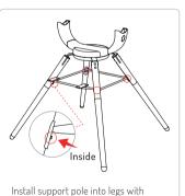
screws M6\*20 and tighten the
