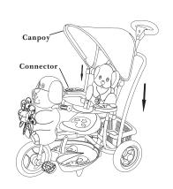
Insert the canopy into the connector as shown by the arrowhead in the picture.
