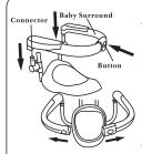
Insert the connector into the safety bar until fixed. (See diagram). Fix the safety bar after your baby is seated. To remove the safety bar, press the button and pull it outwards from both the sides.
