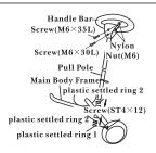
Insert two plastic settled rings into the main body frame, press following the arrowhead direction. Then insert the pull pole into them, and connect the pull pole and the plastic settled ring by the screw (ST4 x 12). Connect and tighten the pull pole and the handle bar by the screw (M6 x 40L), screw (M6 x 35L) and nylon nuts.
