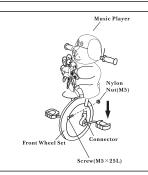
Insert the front fork set into the connector on the front wheel set. Tighten using screws (M5 x 25L) and nylon nuts (both sides). Following the arrowhead direction in the picture, fix the player cap and the player windmill onto the music player sequence. Put two batteries of 5 into the music player and press the button to hear the music.
